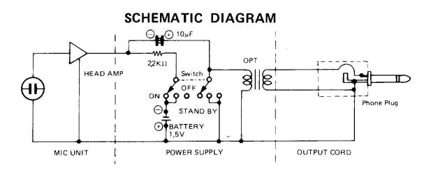
On our own PZMs we have replaced the original (unbranded) ¼" jack plug with a balanced (Neutrik) Male XLR connector, and modified the circuit to use 48V phantom power instead of a 1.5V AA battery. The output of the modified unit is balanced.
